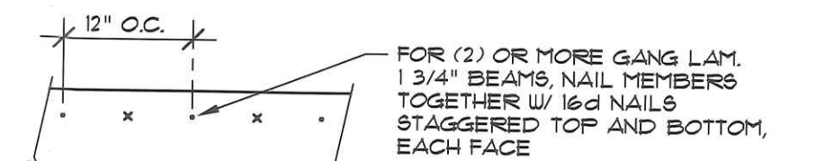
MULTIPLE GANG LAM. DETAIL NOT TO SCALE
