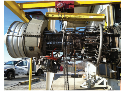
An OMEGA JV2 gas turbine engine is lifted out for repairs
