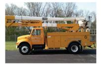
The truck is an International 4900 chassis with a DT466E diesel engine. The boom/bucket has a 55-foot vertical reach, two-man bucket, with a material handler. Service records are available upon request. Dielectric certification was performed on this truck in the fall of 2015. The paint and tires are in very good shape. The truck has been stored inside throughout its entire tenure in the electric department.
