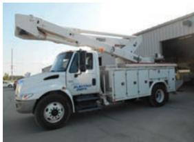
The truck has a fiberglass utility body with aluminum floor, tailshelf body and understructure, and a Versalift VST 6000 material handler.
